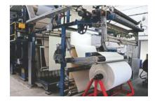
A new sanforizing machine (Monforts) with double rubber cylinder installed.
