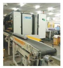
To minimise the manual errors during packaging, we have introduced automated packing machine that can be programmed and monitored through microprocessor interface. This machine works on the functions like auto rolling, cutting, sampling, labelling & palletizing. In addition to eliminating manual errors in marking or weightage, it also saves on the packing time.
