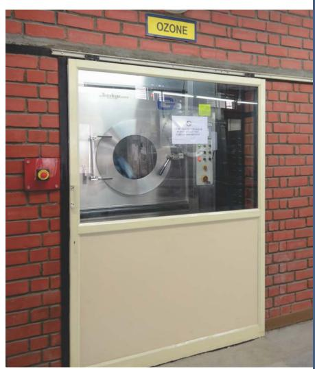
In a conventional softening process, textile products go through a washer containing water and chemicals before being spin dried and tumble dried. Each cycle consumes a huge quantity of water. Keeping in mind our need to rationalise water consumption, we have introduced 'e-Soft technology' at our Bengaluru unit.
